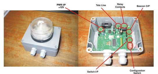
Mode 1 – The beacon will activate when a call is in progress. If the call is answered the beacon will continue to light until the Switch Input has been shorted.
