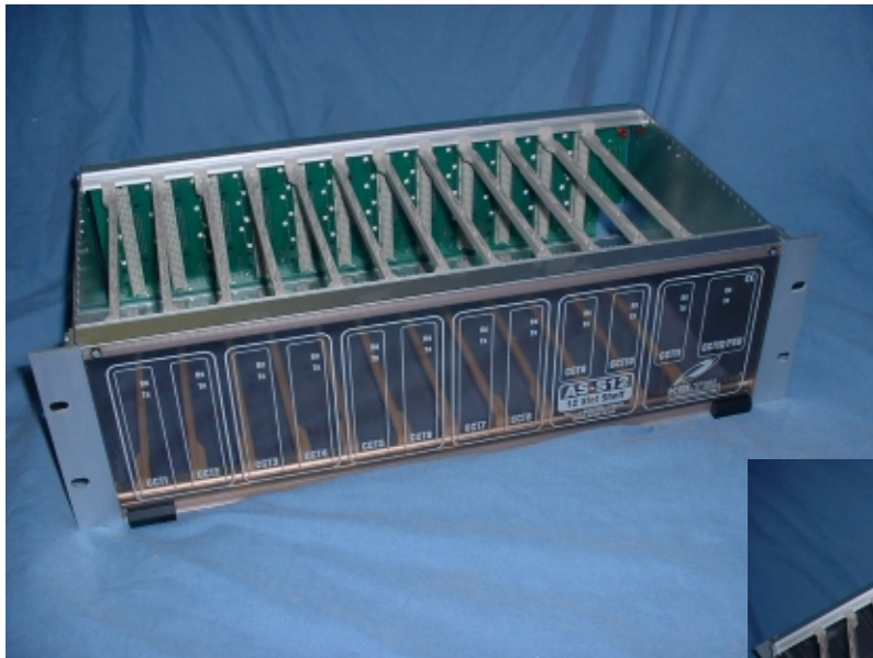
Front View of Hinged Perspex Panel (card guides can also be viewed)
