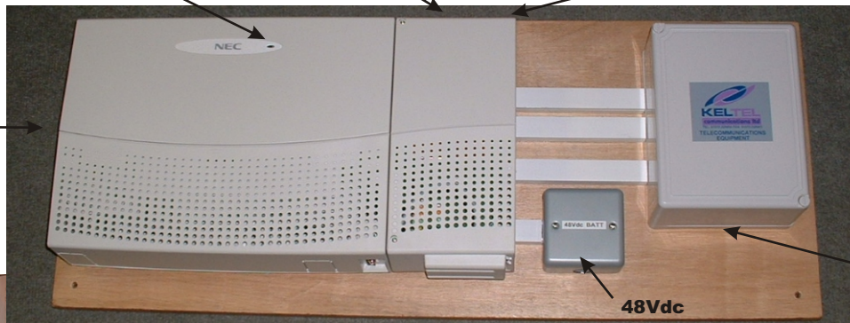
Phone System Status RED/GRN E&M LEDs Yellow 48V LED
