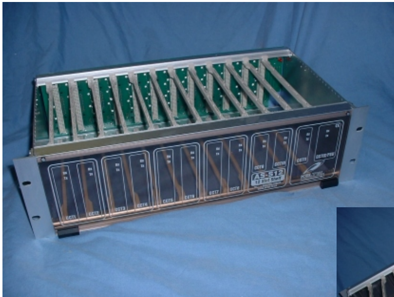
Front View of Hinged Perspex Panel (card guides can also be viewed)
